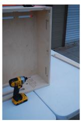
Step 4 – Apply glue to Item #19 (Top Panel) and assemble. Wipe away excess glue. Use a Ratchet Strap to secure the panels together making sure the strap is oriented at least 2" from the front of the cabinet.
